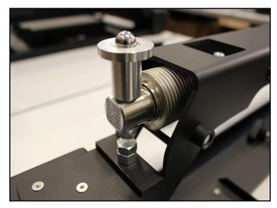
Figure 7 Load cell balls
