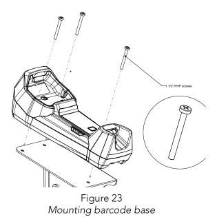
The screws will pass through the mounting holes of the barcode reader stand and fasten to the corresponding holes in the mount.
