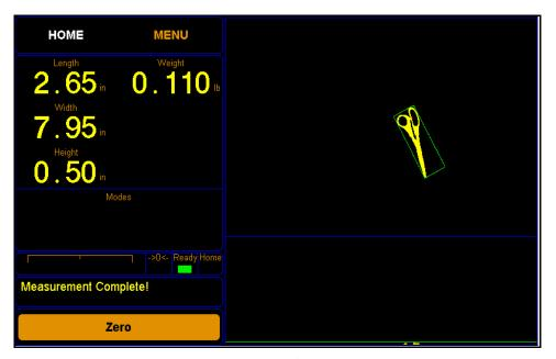
Figure 27 Measuring gate display
