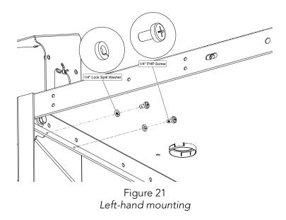
When mounting on the right-hand side of the cart, you may remove the side panel in order to have better access to the bracket mounting holes.
