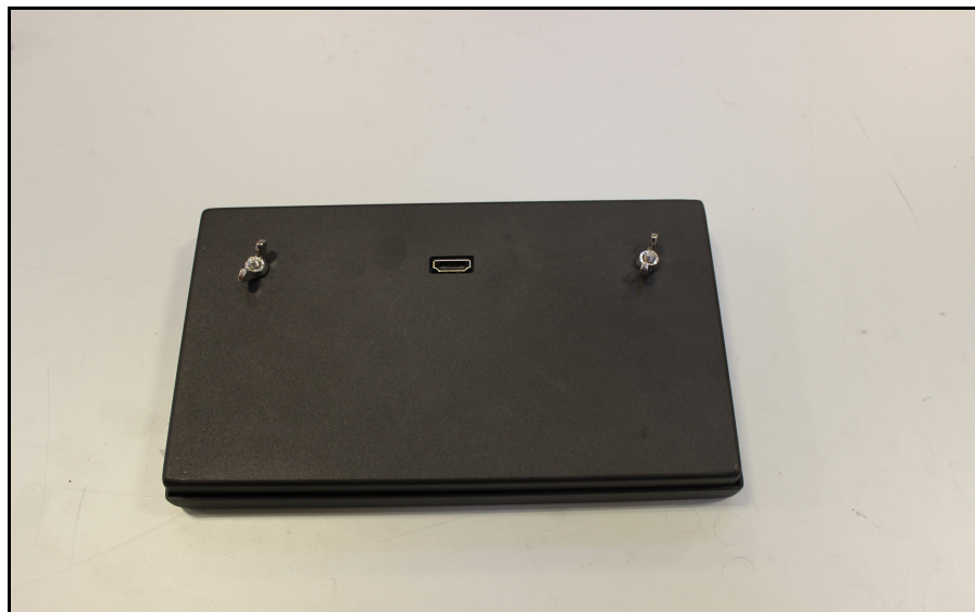
Figure 10 Touchscreen wing nuts
