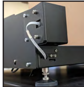
Plug cables into receptors on sensors (D or E), clicking them in place.
