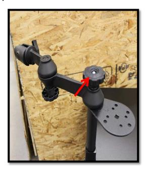
2. Loosen the indicated handle until the swivel arm fits into the cart mount arm. Tighten the handle to secure the swivel arm in place.
