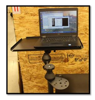
5. Adjust the arms until you are satisfied with the position. Make sure all handles are securely tightened before putting a laptop in place.
