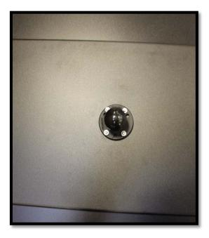
3. Screw the ram mount into the bottom of the laptop tray if it hasn't been attached already.
