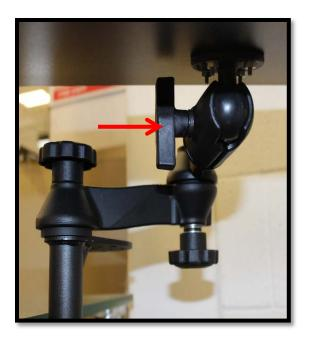
4. Attach the laptop tray to the swivel arm by loosening the indicated T-handle. Insert the tray and adjust it to the desired position.
